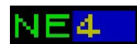
Terminus indicator - in this example, 4 buses are available at the NE (Newport) terminus.
